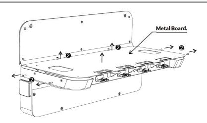
2 Remove the 6x screws and take off the Metal Board.
